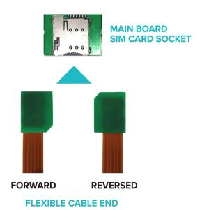
In mock card end (this end will be inserted to the slot of your board), pleaseconfirm the broken corner direction is forward or reverse.
