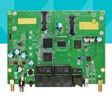
MT7915 Wi-Fi 6 Modules supports  $4\times4$  5GHz reach 2401Mbps. With 2 x MT7915 modules is to be 3 bands backbone mesh router.
